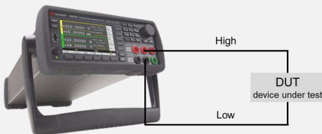
Same measurement using an SMU
